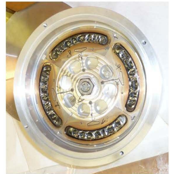
Fig. 7 The ^{249}\text{Cf} target wheel after the bombardment with the ^{50}\text{Ti} beam dose of 1 \times 10^{19}
