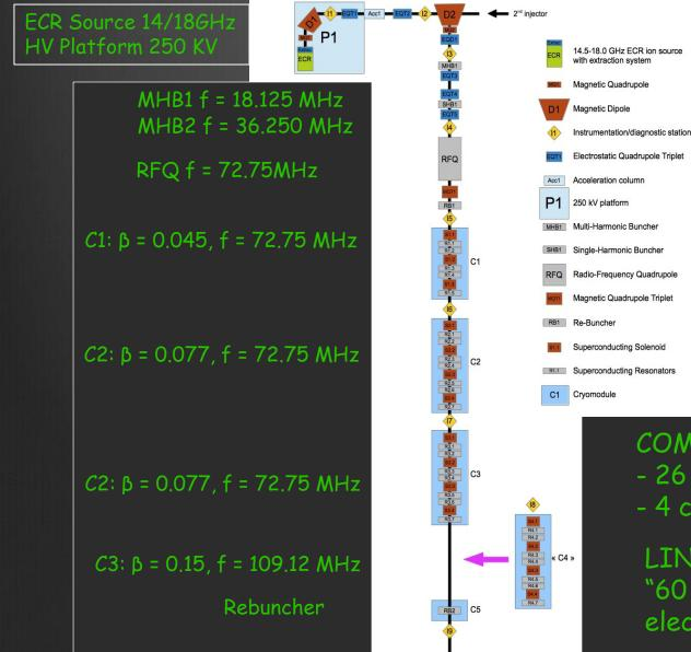
COMPACT DESIGN: - 26 cavities - 4 cryomodules
